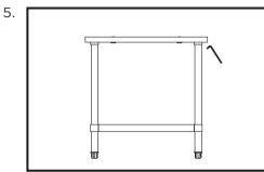
Use 4 x 8mm Allen key screws to secure bench-top section to the legs.
