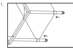
Insert legs through the bottom of the shelf. Locate the scribed mark and position bottom of shelf on the scribe mark.
