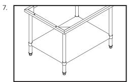
Level the stand by adjusting the adjustable feet on the bottom of the stand.
