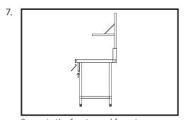
Screw in the front panel from inner corner. (This is an optional asthetic add on)
