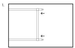
Insert legs through the bottom of the shelf. Locate the scribed mark and position bottom of shelf on the scribe mark.
