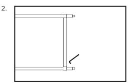
Use 4 x 8mm Allen key screws to secure the shelf section to the legs.
