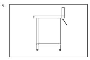
Use 4 x 8mm Allen key screws to secure bench-top section to the legs.
