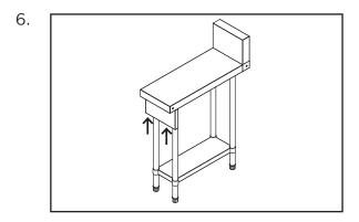
Screw in the front panel from inner corner. (This is an optional asthetic add on)
